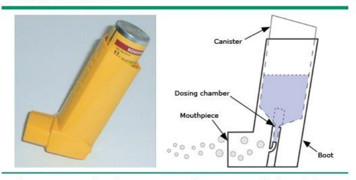
Medication is stored under pressure in the canister and released from the dosing chamber when the canister is pressed downward.
